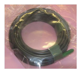
Safety Fuze is used in demolition work where a delay is required to give personnel time to retire to a place of safety before the charge detonates.
